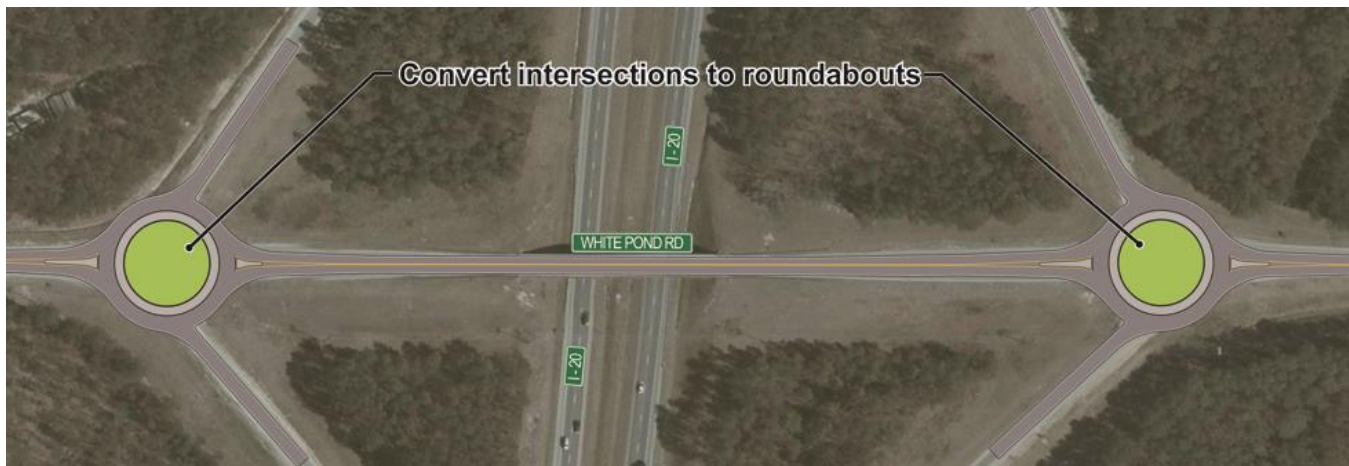
Figure 4.3-2 | Long-term Proposed Improvements for White Pond Road/I-20
